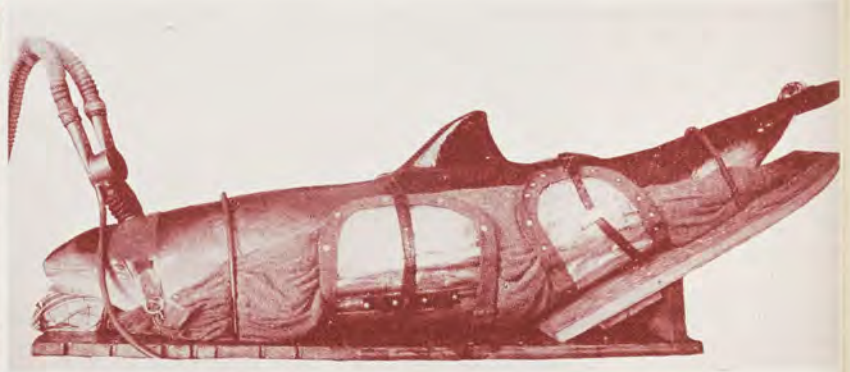
PORPOISE READY TO DIVE, ATTACHED TO RESPIROMETER
